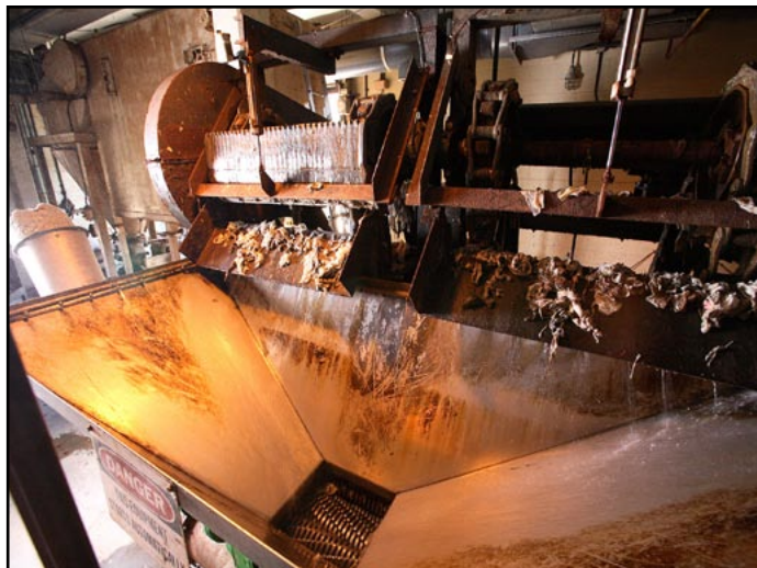
The Screenings Washer Monster, operated by the bar screen motor, collects screenings in this square hopper.
