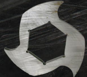
Specially designed three tooth cutters are used with the Fish Cleaning Station.
