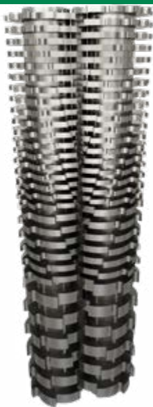
Figure 3. Dual-shaft grinders utilizing custom stacks of varying cutter configurations are better equipped to handle a mix of wastewater debris while improving efficiency and extending grinder longevity. Here, 7-tooth cutters made from abrasion-resistant alloy steel accommodate rocks and heavy debris at the bottom of the wastewater flow, while 17-tooth cutters with special wipe-shredding features break down wipes, diapers, and other floating debris near the top of the flow.
